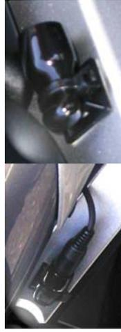
A rubber connector cap and fixings are provided to protect the headset extension cable connector when not in use. The rubber cap can be secured to the bike with the cable tie fixing and cable tie as shown. This provides weatherproof and secure stowage when the headset is not being used.
